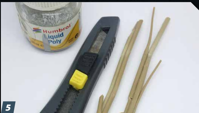
5 Glue the lengths of spruce together with liquid plastic cement. Feel free to bend them into natural-looking shapes, or even heat and stretch the ends to get tapers. Be creative!
