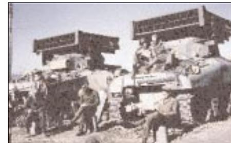
Even when fitted with M17 rocket launchers, these Shermans could also be used as chairs during mail call. Note the differences between the welded (left) and cast hulls. U.S. Army photo
