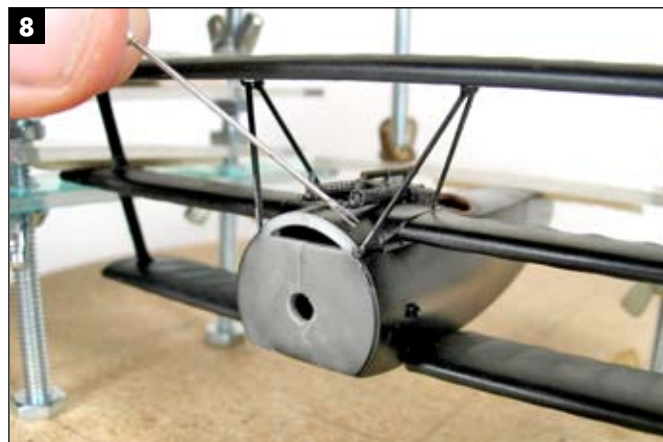
8 With the parts aligned properly, Kevin applied super glue using a large sewing needle. Cut off the top of the loop and it will hold a tiny amount of glue.
