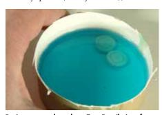
Resin parts, such as these True Detail aircraft wheels, need extra attention to clean off manufacturing residue. Bleche-Wite tire cleaner does the job well, but be sure to wear hand and eye protection — this is strong stuff!
