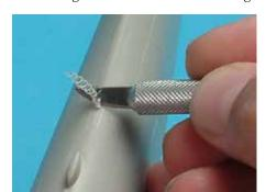
Liquid styrene cement joins pieces by melting the plastic. With judicious clamping, a little plastic will seep out of the join and close the gap; slicing the excess off cuts down on sanding time.
