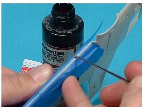
But usually there is some sanding involved in smoothing a filled seam. Here, masking tape protects surrounding surfaces while super glue and accelerator are being applied and during the sanding with follows.
