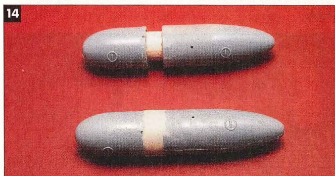
The kit drop tanks were cut in two and lengthened. The tank on top shows the wooden dowel used to maintain correct length. The bottom tank has had the gap filled with epoxy putty.
