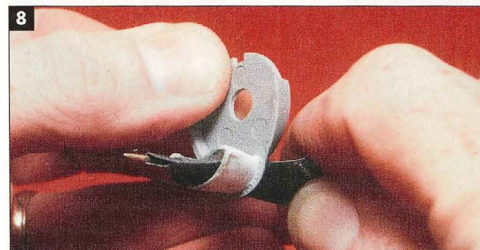
Pat forces 400-grit sandpaper with a straight pin into the corners of the carburetor intake.
