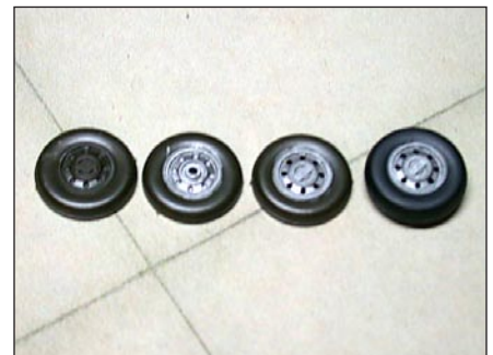
9. I improved the kit's main gear wheels by drilling out the faces.
