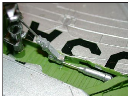
11. The improved retractors now reach the proper spots in the wing and on the struts.
