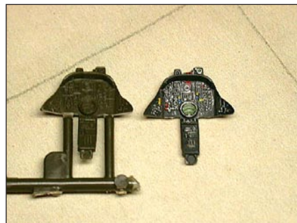
8. I painted the instrument panel flat black and dry-brushed silver to highlight the raised detail. An unpainted panel is on the left.
