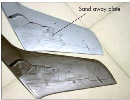
1. Items to be removed included the stiffening plates on the bottom of each wing. I sanded them away and rescribed the panel lines.
