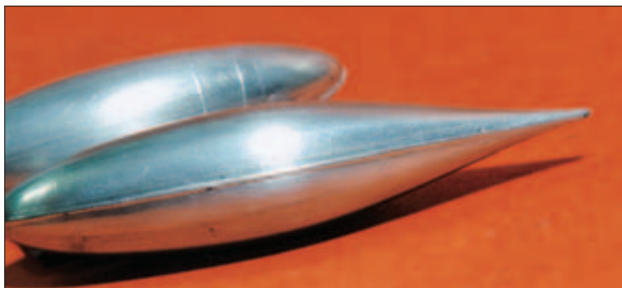
6 Once the covered tank is scoured with 0000 steel wool, the seams between the pieces of foil practically disappear.
