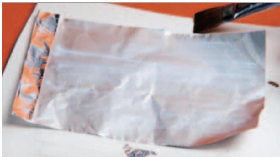
1 If you aren't using Bare-Metal Foil, you'll need to brush Micro Metal Foil Adhesive on the matte side of household aluminum foil. The folded-over edge on the foil sheet serves as a handle.
