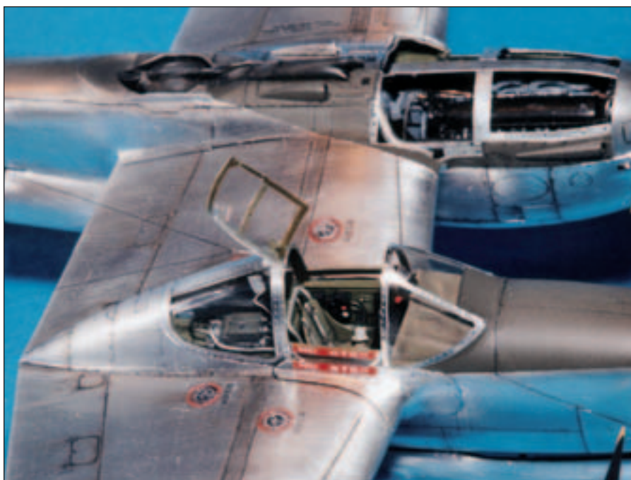
Nothing looks more like aluminum than aluminum. Adhesive-backed aluminum foil is available in many hobby shops, or you can add adhesive to household foil.
