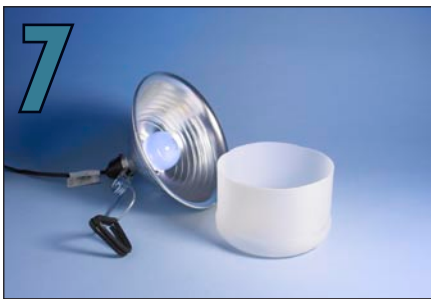
The bottoms of gallon jugs taped to bell reflectors work as diffusers. Daylight-balanced bulbs give natural results (here on a blue background) without a lot of image-editing to correct color balance.
