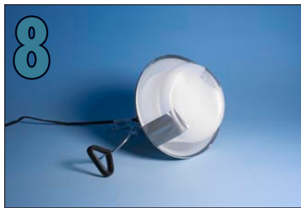
The bottoms of gallon jugs taped to bell reflectors work as diffusers. Daylight-balanced bulbs give natural results (here on a blue background) without a lot of image-editing to correct color balance.
