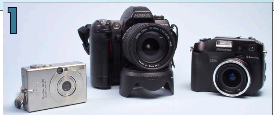
1 The simple, automatic point-and-shoot camera at left is not likely to have manual controls. At right is an example of a mid-level "all-in-one" with a decent selection of controls. This five-megapixel model is a couple of years old now. In the middle is FineScale's DSLR – more than enough control for model photography.
